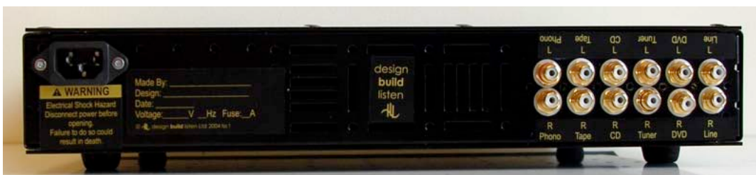
ezChassis as a Preamp. 'Upside-down" with IEC mains socket. Label covers 'speaker' holes
